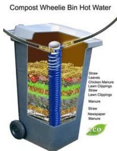
While there, I took a few hot showers where the water was heated by running water hose through a huge compost pile. The internal temperature of decomposing organics heated the water nicely! Here's an [example](#) (left picture) of the principle I found on the internet.
