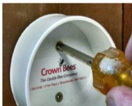
Fig. 2 Tighten upper screw, back out 1 full turn.
